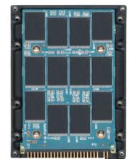
Moreover, with no moving mechanical parts, they can be dramatically faster and more rugged. They require less power, generate less heat and have greater reliability. These factors can lead to improved battery life in a laptop.
